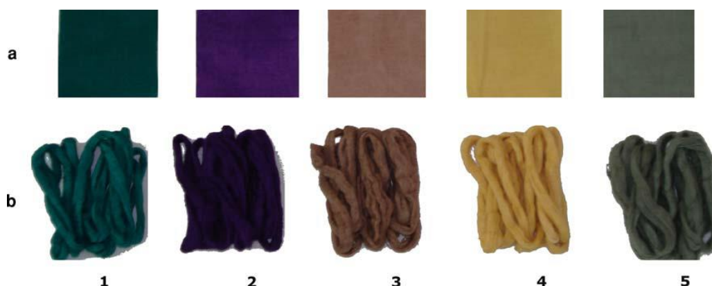
Photograph of dyed samples a) fabric and b) yarn with different vat dyes 1. Green FFB, 2. Violet RR, 3. Brown BR, 4. Yellow RT, and 5. Olive R
